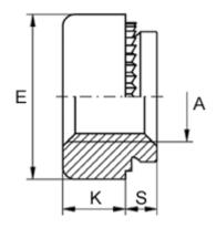
Female thread A = M3Height K = 2.0Max recess height = 1.0Min distance to edge = 4.0Outer diameter E = 7.0Plate thickness = 1.5 to 2.3
